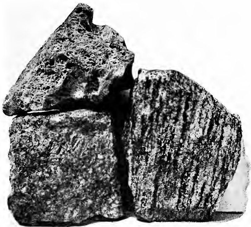
FIG. 23. — The banded appearance of gneiss (on the right), in contrast with granite (on the left) and pumice (above).
